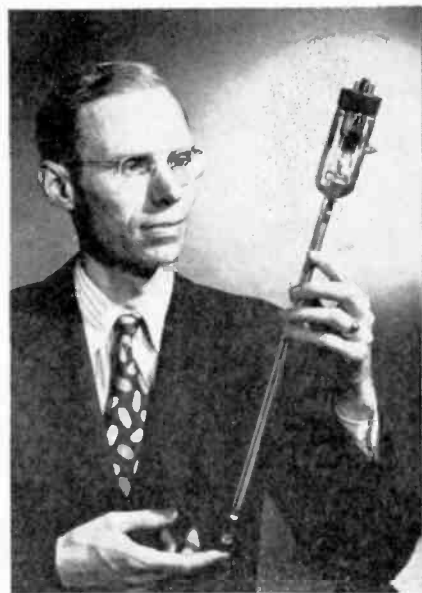
Dr. John R. Pierce of Bell Labs holds new amplifier tube with a power gain of 10,000 over a bandwidth of 800 mc. Tube is designed to operate in the 5000-mc region.
